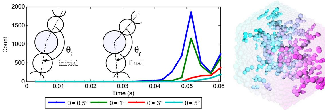
Fig. 6. (Left) The number of particles in buckling force chains which buckle by no less than the threshold value of  $\theta$ ,  $\theta_b \geq \theta$ , for one time step in the simulation. Inset illustrates the buckling angle  $\theta_b = \theta_i - \theta_f$ . (Right) Buckling force chains at simulation time of 0.0606, where  $\theta_b \geq 1.0^\circ$ : a total of 627 particles are in this set.
