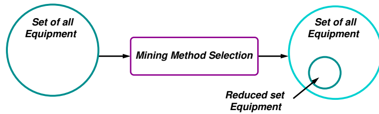
Figure 5 Mining method selection is the process of choosing a particular style of mining, e.g. open-pit, dredging or stripping. Once the method is chosen, the set of equipment to choose from is reduced. Heuristic or exact methods can then be applied to choose the fleet.
